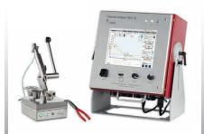
Thermal Analysis **TA 12.13** for determination of grain refinement and modification for the evaluation of mechanical properties
