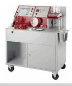
**ALSP highline** incl. crucible pre-heating chamber for determination of grain refinement and modification for the evaluation of mechanical properties
