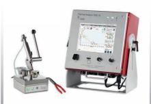
Thermal Analysis **TA 12.13** for determination of grain refinement and modification for the evaluation of mechanical properties
