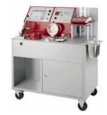
**ALSP highline** incl. crucible pre-heating chamber for determination of grain refinement and modification for the evaluation of mechanical properties
