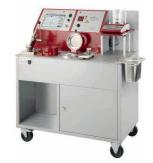
**ALSP highline** incl. crucible pre-heating chamber for determination of grain refinement and modification for the evaluation of mechanical properties
